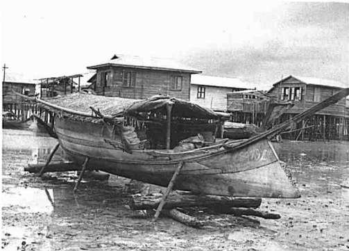
7 Careened lepa showing roofed living quarters, carved bowsprit, poling-platform, and ia'am .
