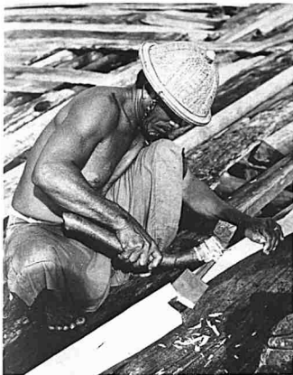
9 Constructing a new lepa ; an adze is used to shape the bengkol .
